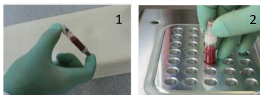
Figure 6-1: Mix by inverting each TC tube gently (1). Place TC tubes in the incubator (block) (2).
