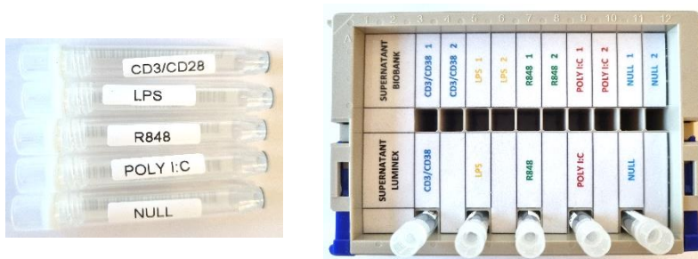
Figure 6-2: Matrix tubes labeled with stimuli labels and placed in the matrix work box (supernatant for Luminex).
